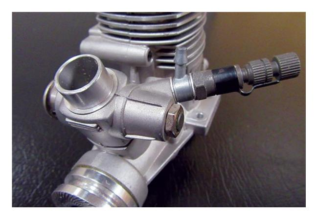
A typical carburetor has two needle valves to adjust the fuel/air mixture. The high-end needle assembly is shown here.
