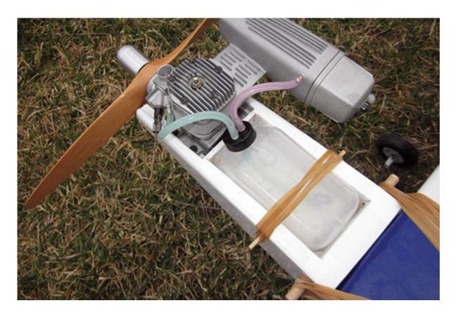
When attaching the fuel line and vent line from the fuel tank, make sure that they are not kinked or resting against the engine.
