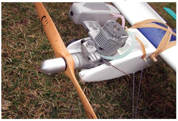
Glow engines need to be installed on your airplane with a strong, rugged mounting system. Your propeller should be the recommended size and properly balanced. Notice the wire extension added to the main needle valve to keep fingers clear of the propeller.
